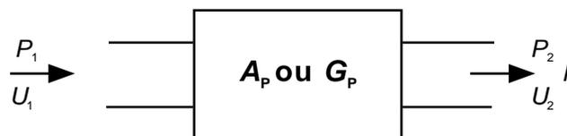
$$\text{Soit : } A_p = \frac{P_2}{P_1} \quad \text{ou} \quad A_U = \frac{U_2}{U_1} \quad \text{ou} \quad A_I = \frac{I_2}{I_1}$$
